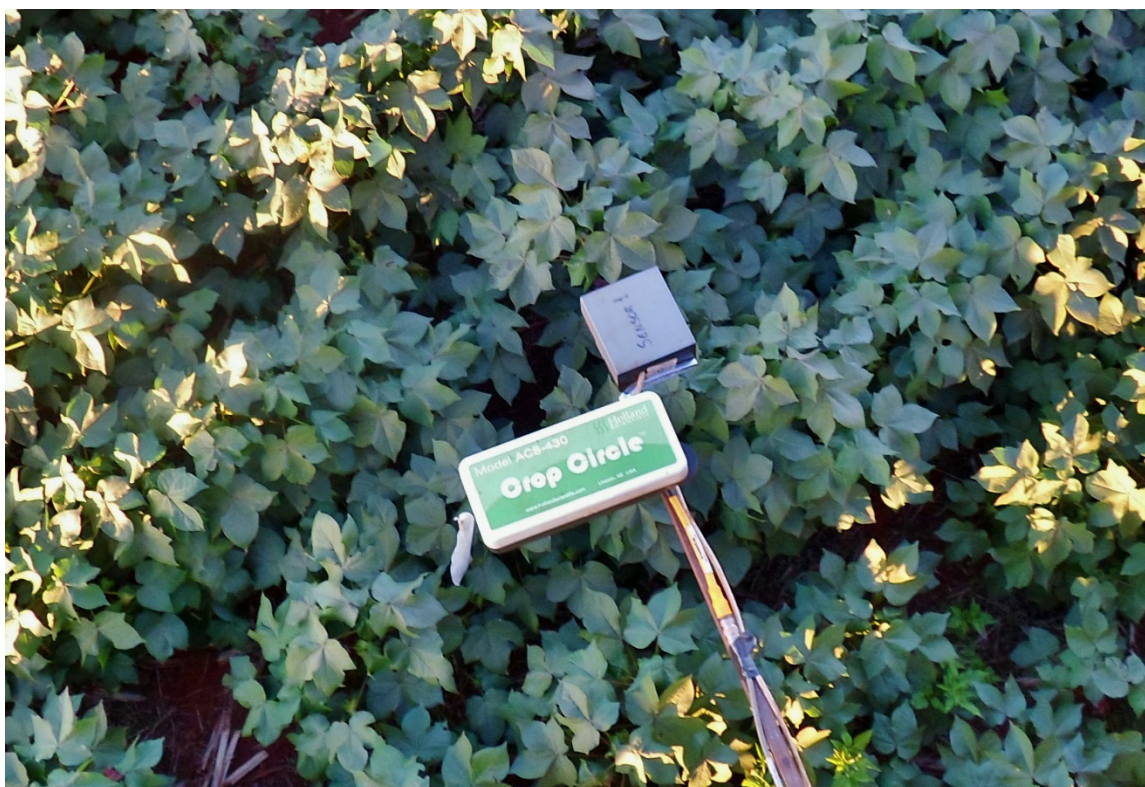
Figure 1. Positioning of sensors above narrow row cotton canopy.
