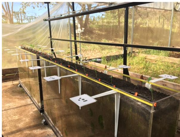
**Figure 2. Bar codes used to overlap and geo-reference the images**
