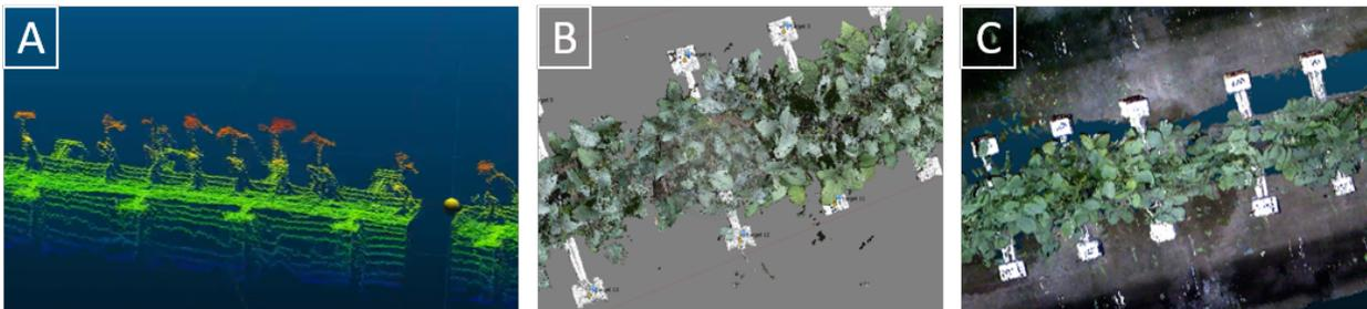
Figure 3. Examples of point cloud obtained with: a) LMS -200 b) T3 Canon and c) Kinect V1
