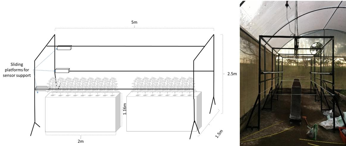
**Figure 1. Structure assembled to support the sensors.**
