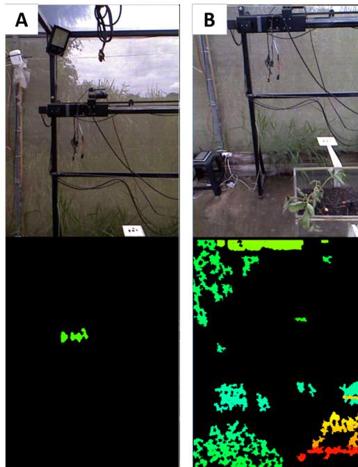
Figure 4. RGB (top) and depth (bottom) images from K1 on a very intense sunlight exposure (A) and on a less intense sun light exposure (B)
