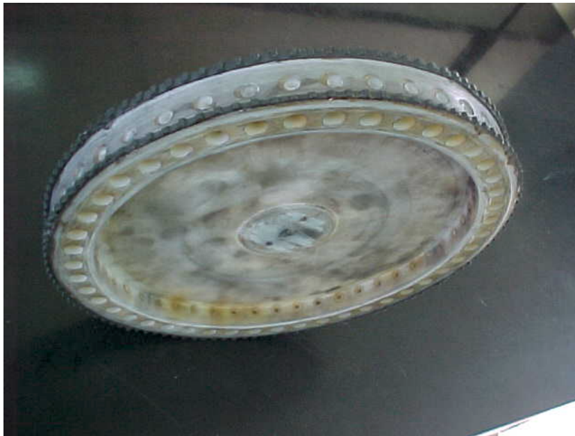
Figure 2. View of the seed metering nylon ring with 45 radial cells.
