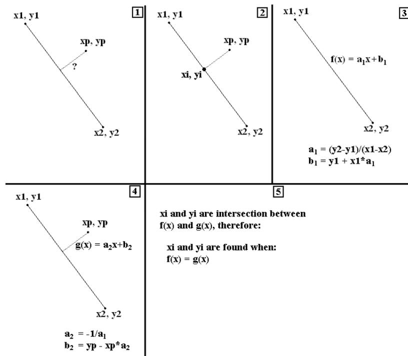
Fig. 3. Steps used to retrieve the distance between a line and a point.
