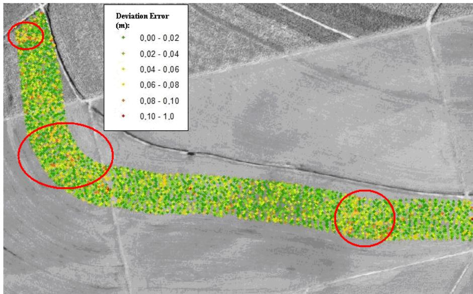
**Fig. 5.** Map view of the deviation error of the harvester on the field.
