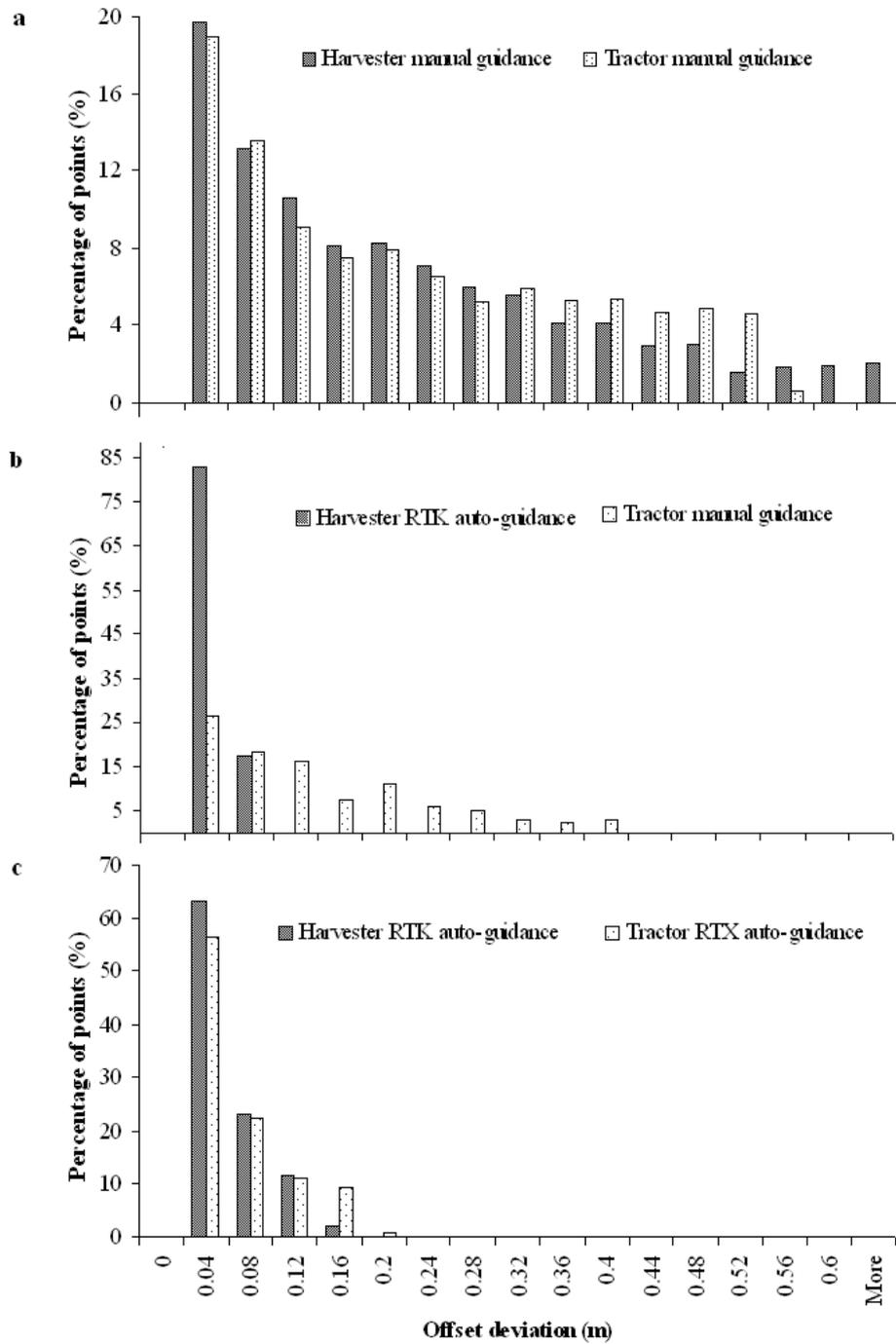
Fig. 6. Offset deviation of a harvester and a tractor-carrier in three distinct guidance scenarios.
