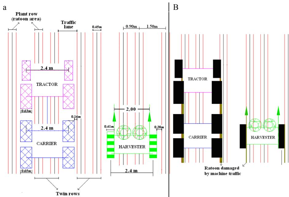
**Fig. 2.** Scale dimensions and of lanes and machine width properties (in “a”) and damage of sugarcane ratoon in case of the offset of the machines (in “b”).
