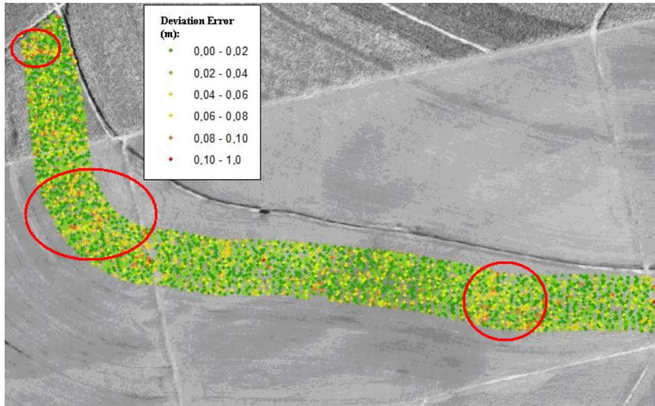
**Fig. 5.** Map view of the deviation error of the harvester on the field.
